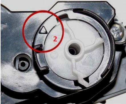
Make sure the black arrow on the cover is aligned with the white arrow marked #3 on the TN2210 (low) gear.
