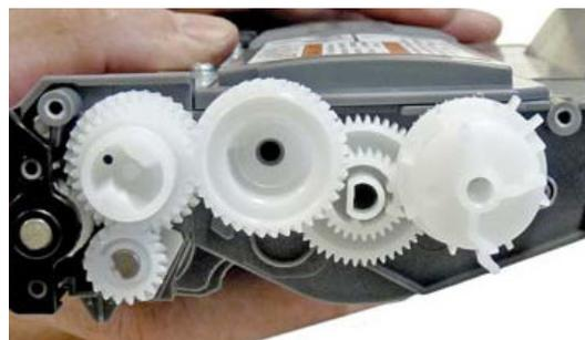
Remove only the white reset gear. Set the reset gear spring as shown
