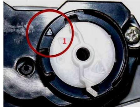
Make sure the black arrow on the cover is aligned with the white arrow marked #1 on the TN2220 (high) gear
