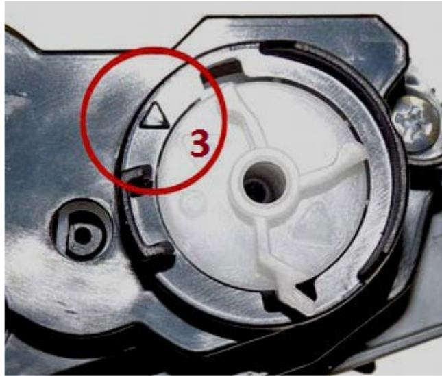
Make sure the black arrow on the cover is aligned with the white arrow marked #3 on the TN2010 gear.
